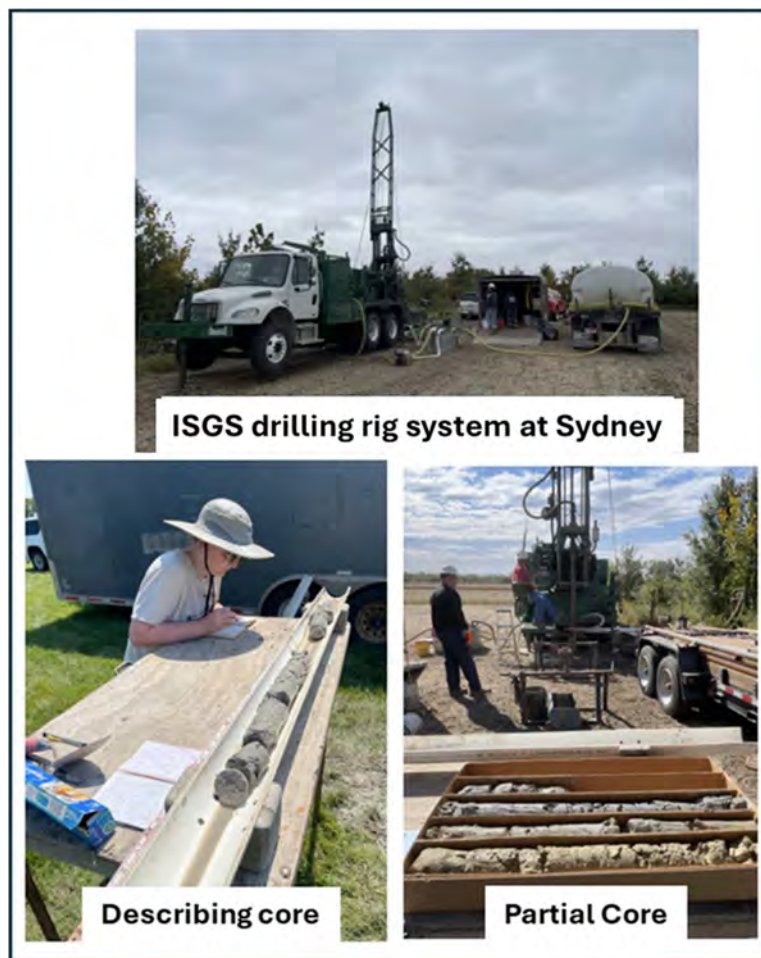
Figure 9. Photos of drilling and core/sample analysis in Sydney, Illinois. Core samples were collected for analysis from surface to a depth of 77.72 m in Flatville and 60.35 m in Sydney.
