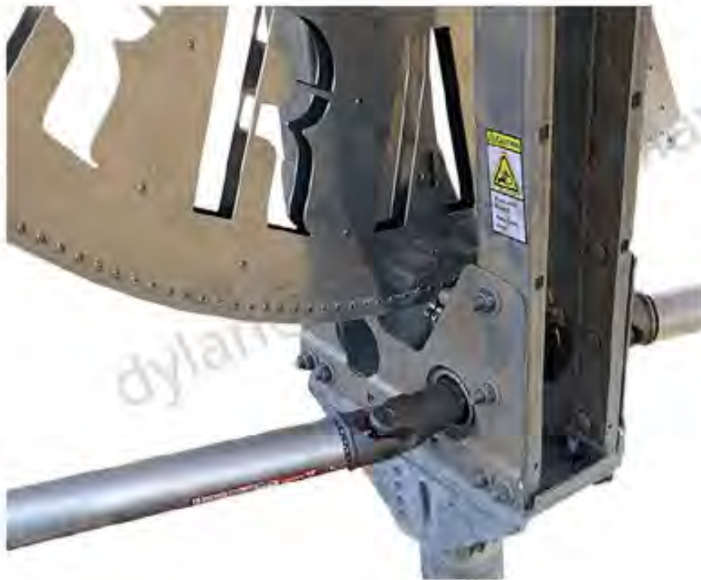
Figure 8-1: Universal Joints in Drivelines
