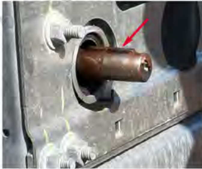
Figure 8-5: Key Located On Shaft
