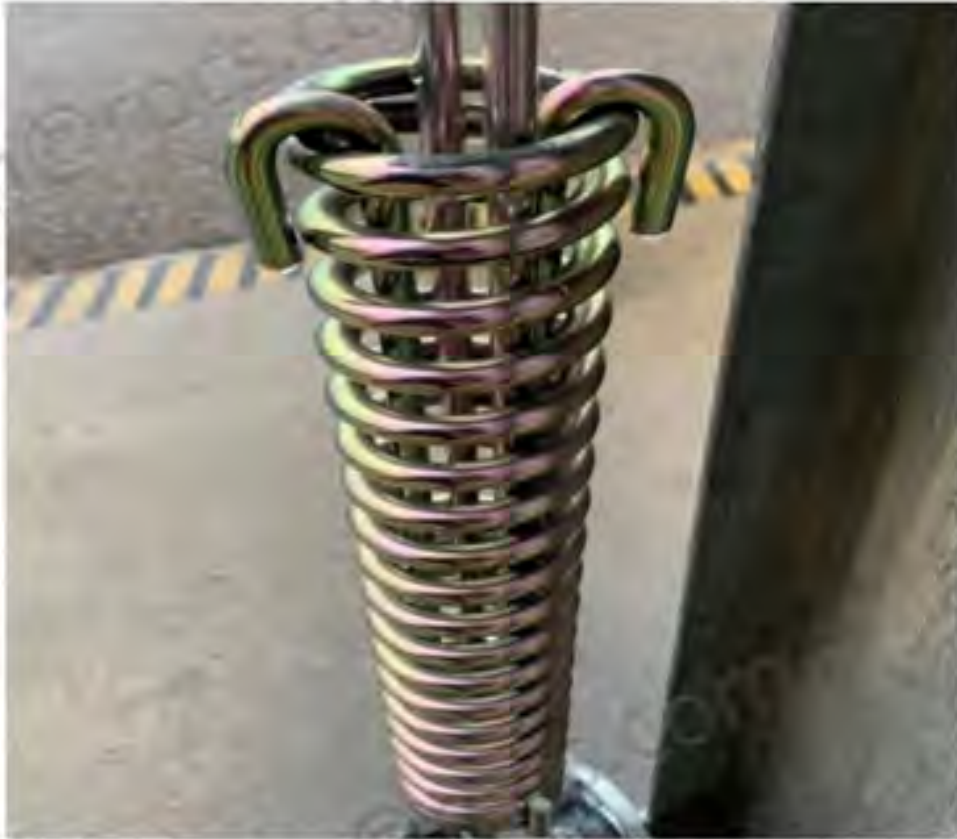
Figure 9-5: Drawbar Hooks Correctly Outside Spring
