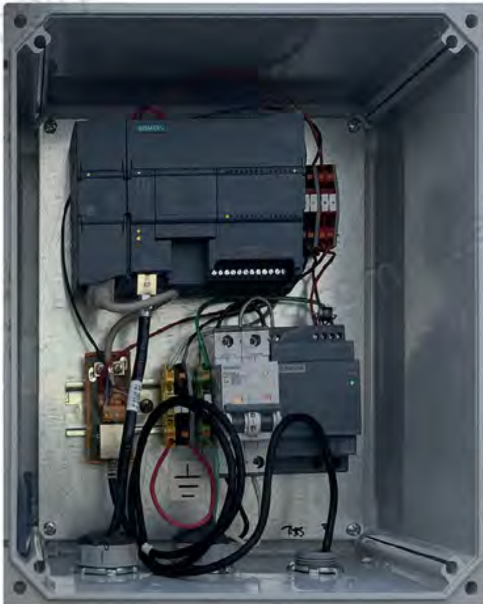
Figure 10-10: Example Site Data Controller Enclosure Interior (US)
