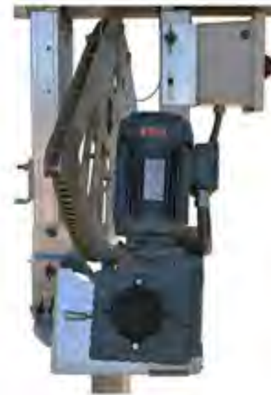
Figure 8-3: Begin Driveline Install At The Motor
