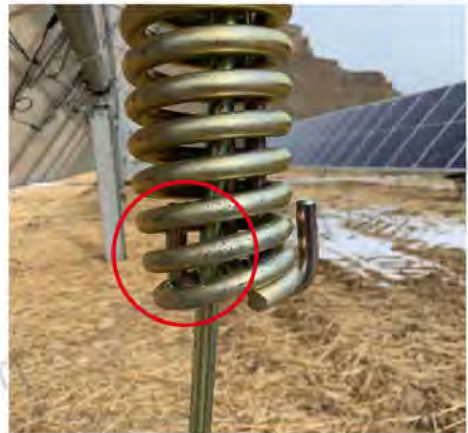
Figure 9-4: Drawbar Hook Incorrectly Inside Spring
