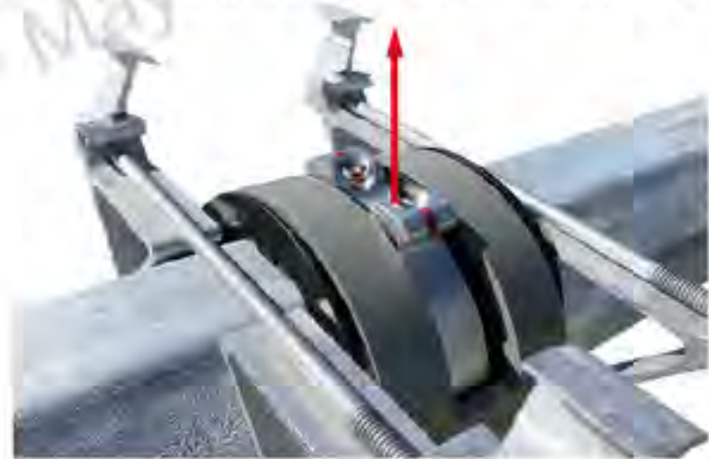
Figure 5-30: Bearing Stop Orientation Check
