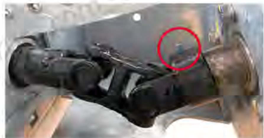
Figure 6-6: Set Screw On Double U-Joint
