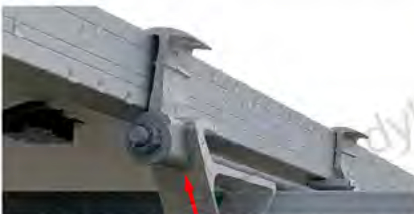
Figure 7-9: Verify Ears Are Flush With Clamp Body
