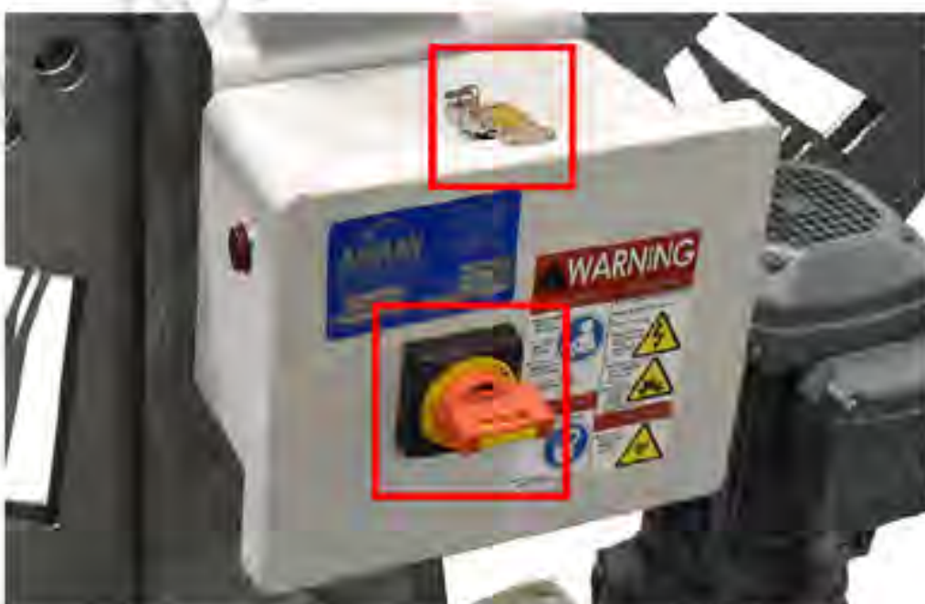
Figure 2-5: Motor Electronics Assembly Lockout Locations
