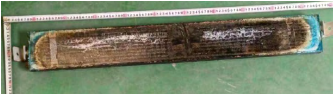
Figure 0-2 – CBFAD Cell After Thermal Runaway
