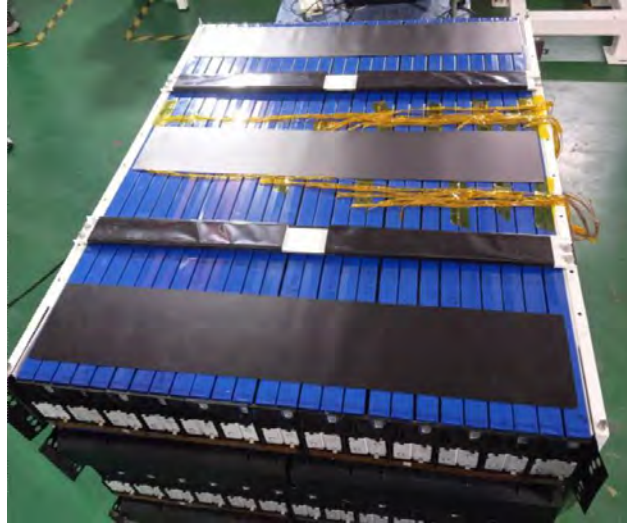
Figure 0-3 – MC Cube Module Assembly
